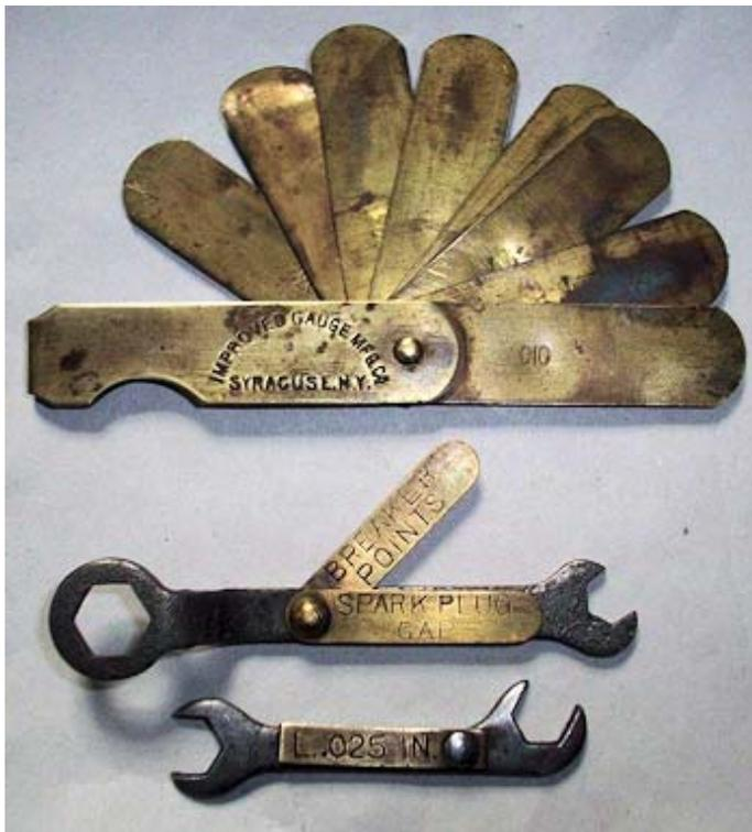
This picture shows a brass gauge made by "Improved Gauge Mfg. Co.", and 2 ignition wrenches with brass leaves. I don't know what engine the middle wrench is for or why you would need the sparkplug gap leaf to be
