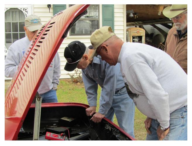
The distributor cap was removed and the points checked out. A dwell meter was hooked up and the dwell checked out with the hot wire in place to allow the engine to start. The battery was then charged to full capacity just to make sure it was up to the task. The Corvair still would not crank without the hot wire in place.
