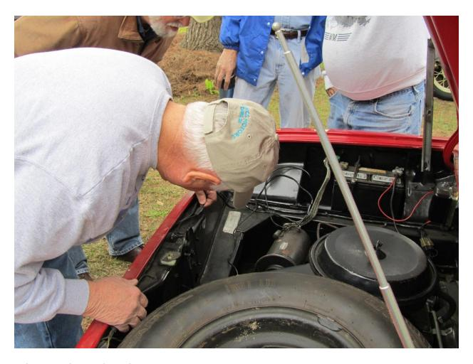
A jumper wire, or 'hot wire' as known by the former juvenile delinquents in the group, was attached from the battery to the hot side of the coil. This allowed the Corvair to start and run just fine. Something was happening in the wiring, connectors or ignition switch to starve the ignition circuit of vital electrons.
