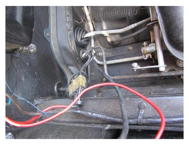
Bill O. promised to pick up some contact cleaner at NAPA and do a proper cleaning of the connector. We are confident this will result in a proper 12 volts making it to the coil and the Corvair should be back to consistent cranking.
