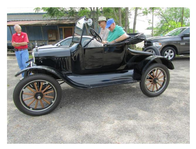
Even with Kevlar bands installed in the 1922 Model T, the student drivers took their toll. A short pit stop was required to adjust the band tension before the lessons could continue. Luckily, everyone was an expert on band adjustment from the first part of tech. day.
